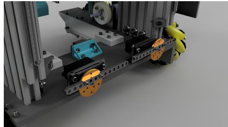
Horn from REV. to pull the foundation we position the robot perpendicularly to it, driving the robot to its edge and then, using the servomotors that grip the foundation, we pull it by simply moving our robot.
