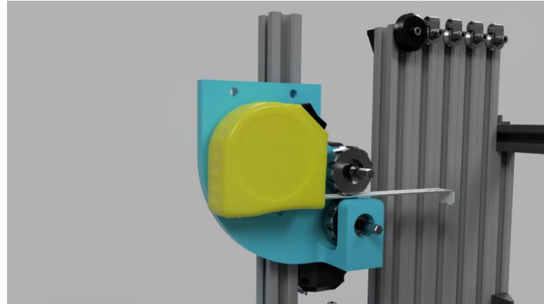
is tied to the motors axis while the other one is freely rotating on an ax fixed with two bearings. The tape measure extends backwards because at the end of the match, when we need to park, the robot is positioned with its back headed to the parking area.
